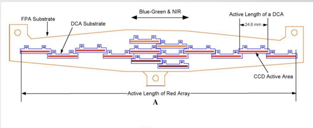
CCD charge transfer Time Delay Integration (TDI) greatly improves SNR
